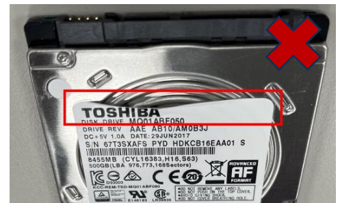
(2) 原廠標籤變形或被撕開 (Label deformed & lifted)
