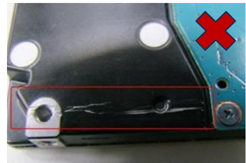
(10) 金屬外殼刮傷 (Covering scratched)
